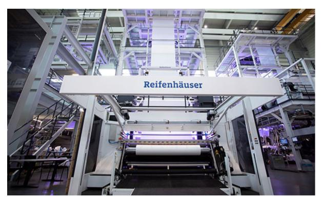
Breathable film protects against infections but allows air exchange which is vital for hospital workers who must wear coveralls for long periods of time. Breathability comes from the pore structure in the material which is produced by a special calcium carbonate addition followed by a stretching process (Reifenhäuser EVO Ultra Stretch).
