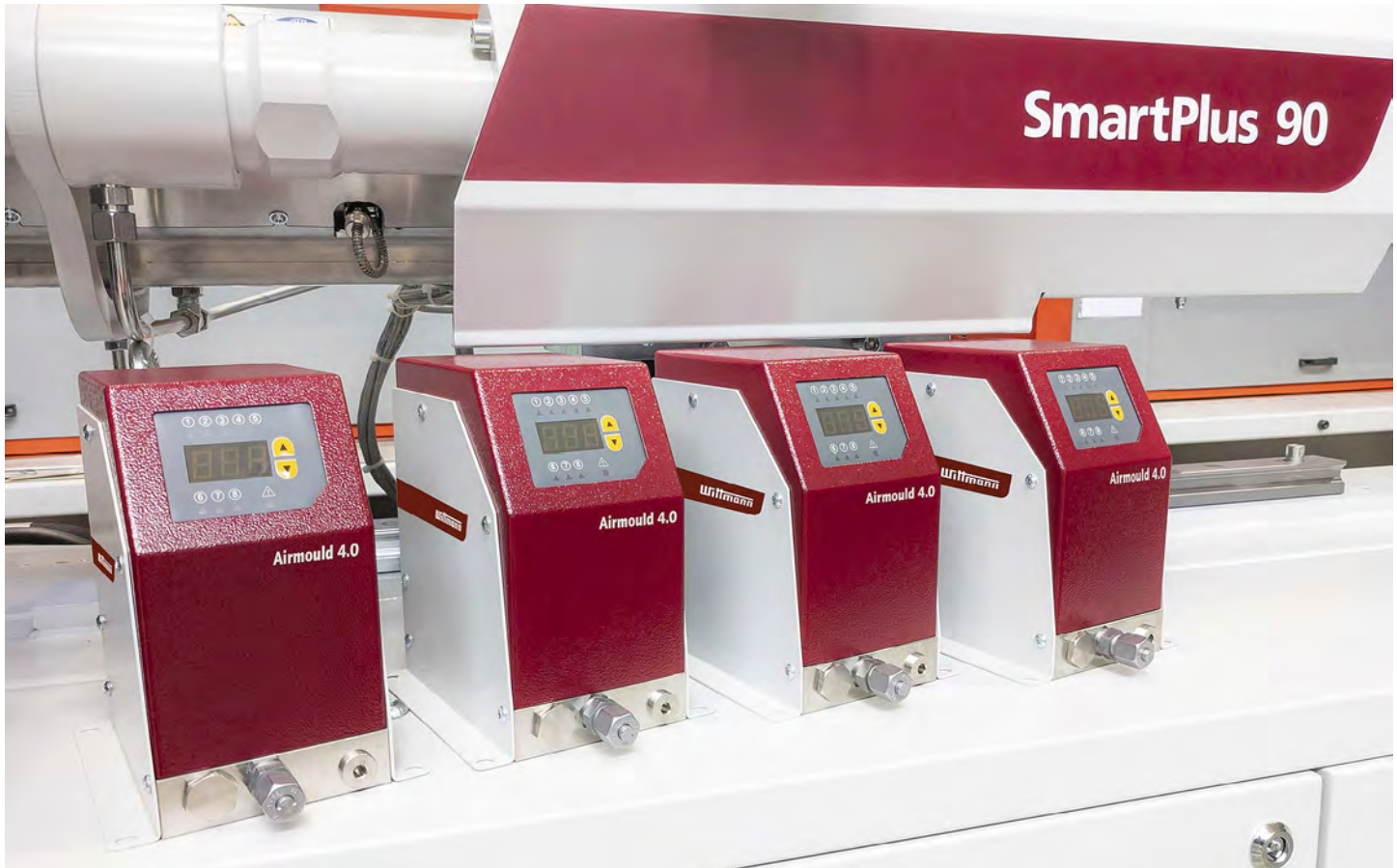
Airmould 4.0 modules, small and directly on the injection molding machine.
