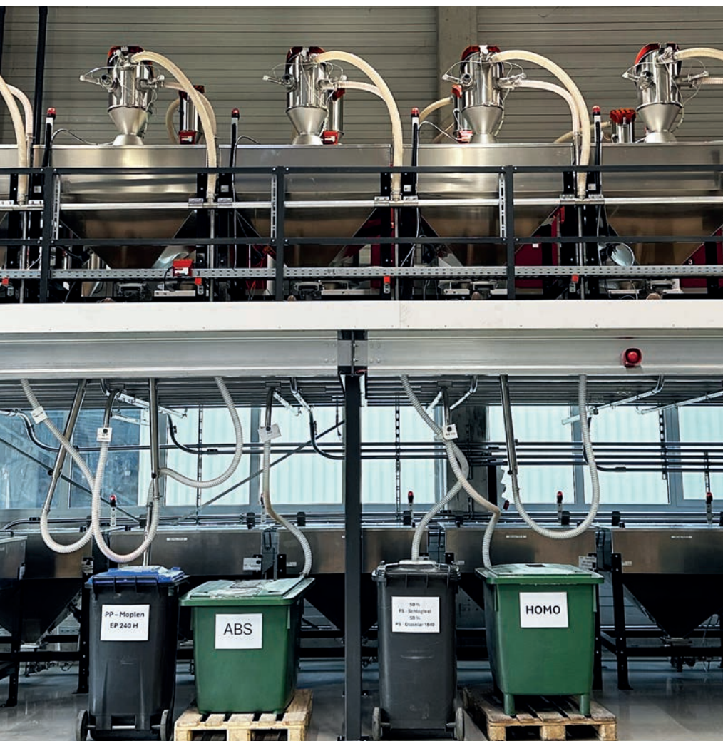
The dryer platform provides a view across the material storage area. The space directly under the platform is reserved for containers filled with the most frequently used materials.
